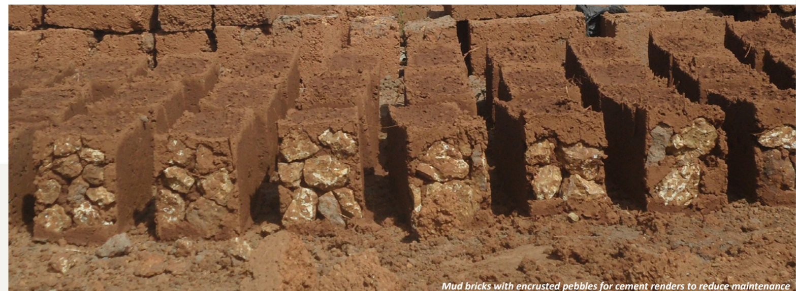
Mud bricks with encrusted pebbles for cement renders to reduce maintenance
